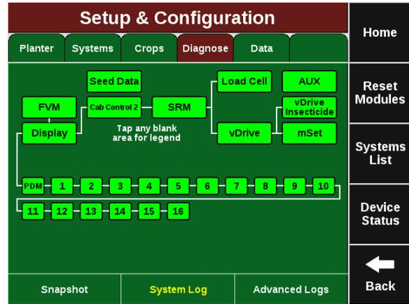
Green - the system is working correctly and communications are good.
