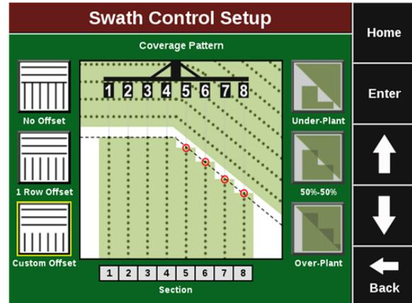
On the left hand side of the screen select a Row Offset. This is the distance from the headlands that seeds start and stop. On the right hand side of the screen select a coverage pattern. This is used when rows are tied together in swath sections.
