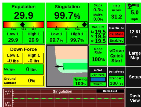
**Note:** The vDrive Quick Start button must be added to the home screen before it can be used. See the 20/20 Operator’s Guide for information on configuring the home screen.
