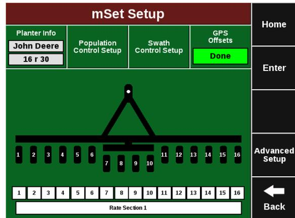
The bottom boxes under the planter indicate the Rate Sections that have been configured and what rows they correspond to.
