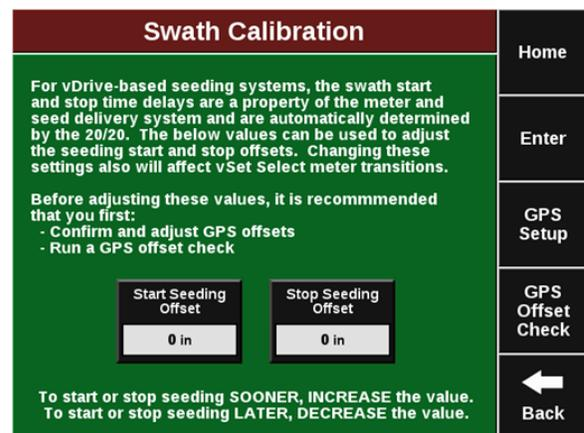
Adjust the Start Seeding Offset to change where the system will begin dropping seeds. Find the distance from where the seeding is actually starting to where it should start by digging. Enter this distance in inches. Negative numbers will move the seeding backwards while positive numbers will move it forwards. Do the same with the Stop Seeding Delay for where the seeding should stop.
