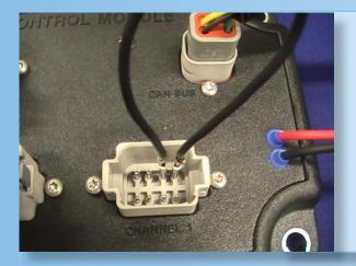
b. If jumping these pins increases the Flow Meter Pulse Count value, then you most likely have an issue with the Control Valve/Flow Meter cable.
