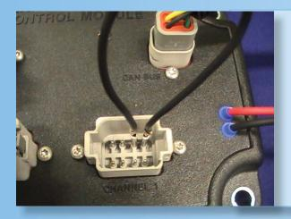
a. If jumping the flow meter connection does not increase the Flow Meter Pulse Count value. trace back to the Liquid Product Control Module and jump pins 3 and 4 (signal and ground) on the Channel 1 port. Make sure you are creating a pulse effect between the two pins by repeatedly removing and inserting one of the pins.
