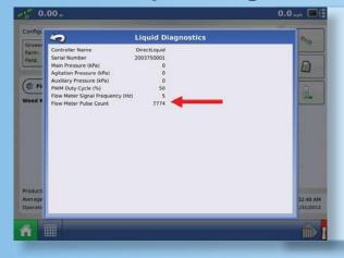
Watch the value for Flow Meter Pulse Count. With product flowing through the flow meter this value should count up. It should count up regardless of the Master Switch being On or Off.
