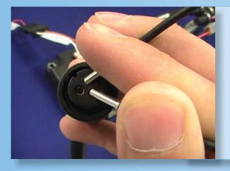
b. If the Flow Meter Pulse Count value increases then you most likely have an issue with your flow meter. If not, continue to step 3.
