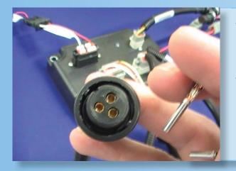
a. Jumping these two pins, you should see the Flow Meter Pulse Count value increase. The value won't necessarily increase by a specific amount. You merely want to see an increase. Make sure you are creating a pulse effect between the two pins by repeatedly removing and inserting one of the pins.
