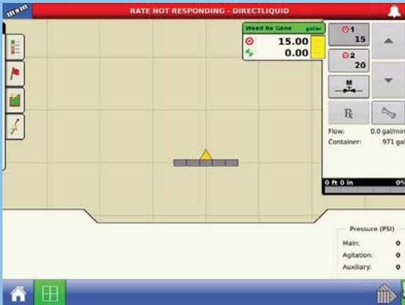
At this point you should be in Rate Not Responding Mode (to the left) and sending voltage out to the control valve to open it. If the screen is flashing Rate Not Responding but the control valve isn't opening, continue to step 8.
