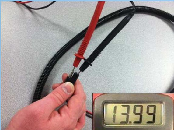
a. Unplug the 2 pin connector from the control valve and test for power while, "Rate Not Responding" is flashing on the monitor. There should be 12 volts present assuming the Valve Response 1 setting is at 100%. If you have power here and the valve won't respond, you have a valve issue. If you don't have power here, continue to step 9.
