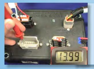
a. Now test for power at the Boom port on the Liquid Module. You'll test for signal on the pin to the corresponding boom (Boom 1 to 1, boom 2 to pin 2, ext.) and use a common ground. If you get 12-14 volts here you most likely have an issue with your Boom cable. If not, continue to step 10.
