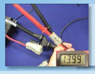
a. If you don't have voltage at the Boom port you'll want to check for power coming into the Liquid Module from a High Current plug. If you have 12-14 volts here you most likely have an issue with your Liquid Module. If not, trace back for power at the battery.
