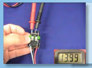
a. You should get 12-14 volts across B & C at this connection. If you are and the boom valve won't open, verify that you have power across pins A & B (power and ground). Without 12-14 volts across A & B the valve can't open. If you have power across B & C and A & B the issue must lie with the boom valve.
