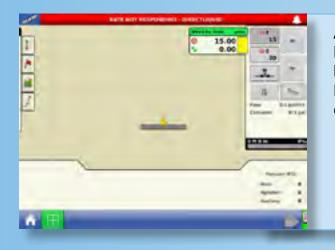
At this point you should be in Rate Not Responding Mode (to the left) and sending voltage out to the booms to open them. If the screen is flashing Rate Not Responding but the booms are not opening, continue to step 8.
