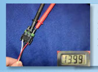
b. If you don't get 12-14 volts across A & B, you need to make sure you have the High Current connection on the boom cable plugged into a High Current plug to supply power to the boom valves. If you don't find power across C & B, continue to step 9. If you don't find power across A & B continue to step 8c.
